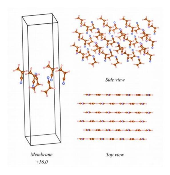
Structure of the acrylonitrile-based membrane following optimization in vacuum at the PBE-D3 level of theory. The optimization of the membrane structure was done using an energy cutoff 700 eV and a 9x9x1 k-point mesh. The energy of the membrane relative to the Pna21 phase of the acrylonitrile ice is given in the figure in kJ/mol acrylonitrile. Credit: Science Advances, doi: 10.1126/sciadv.aax0272
