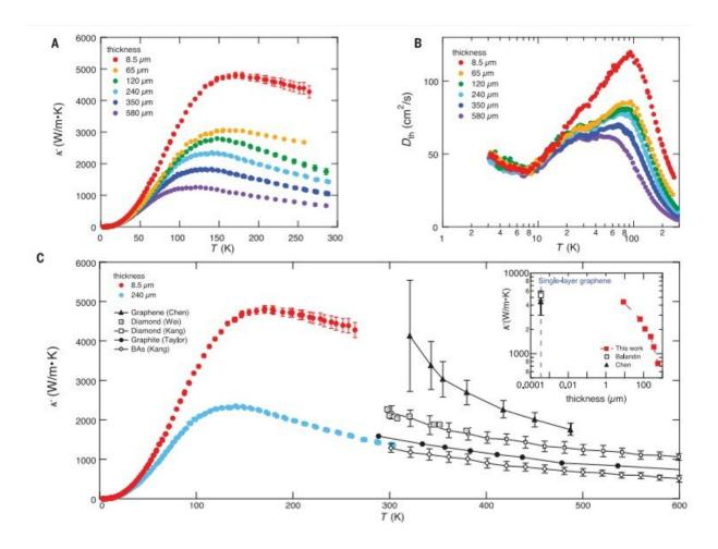
Thickness dependence of thermal conductivity. (A) Temperature dependence of in-plane thermal conductivity k for various sample thicknesses. In the thinnest sample, k attains the largest value (~4300 W/m·K) known in any bulk system near room temperature. (B) Temperature dependence of thermal diffusivity Dth
