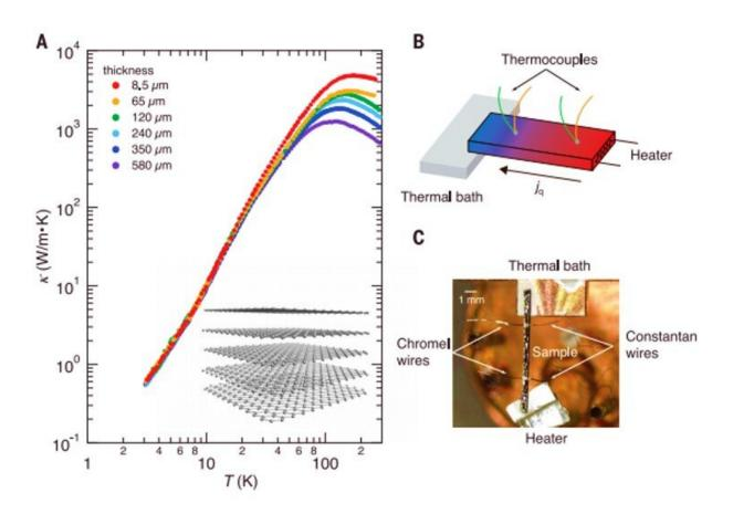
Thermal conductivity and experimental setup. (A) Temperature dependence of in-plane thermal conductivity of graphite with thicknesses ranging from 580 to 8.5 mm on a logarithmic scale. Inset shows side view of the crystal structure of graphite. A schematic illustration (B) and a photo (C) of the measurement setup for the thermal conductivity. Heat current (jq) generated by a heater on one end
