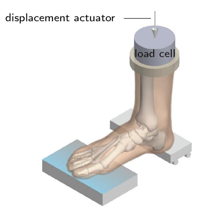
Schematic showing bending test on a human cadaveric foot. Credit: M. Venkadesan
