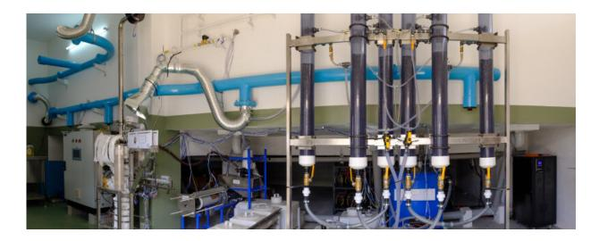
The treatment hardware for the prototype sanitation system that underwent field testing at a textile mill in Coimbatore, India. Credit: Shamsheer Yousaf
