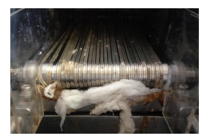
This conveyer of rubber bands separates solid and liquid waste effectively in an experimental sanitation system at a test site in India. But at a facility in South Africa, where the culture uses toilet paper, the results aren't as good. This was one of many lessons learned from two eight-month-long field trials for sanitation systems sponsored by the Bill and Melinda Gates Foundation. Credit: Brian Hawkins, Duke University
