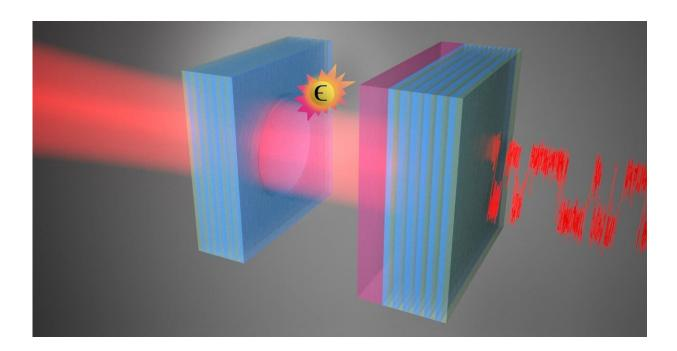
An optical cavity with a nonlinear material (purple) between two mirrors (blue). Light that enters from the left, resonates inside the cavity. Due to noise, the output on the right switches randomly between two values. A small perturbation in the cavity (like a particle, shown here as the yellow  $\mathcal{E}$ ) changes the switching output pattern. Credit: Rodriguez and Boluijt, AMOLF
