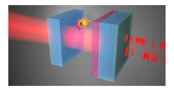
An optical cavity with a nonlinear material (purple) between two mirrors (blue). Light that enters from the left, resonates inside the cavity. Due to noise, the output on the right switches randomly between two values. A small perturbation in the cavity (like a particle, shown here as the yellow  $\mathfrak E$ ) changes the switching output pattern. Credit: Rodriguez and Boluijt, AMOLF
