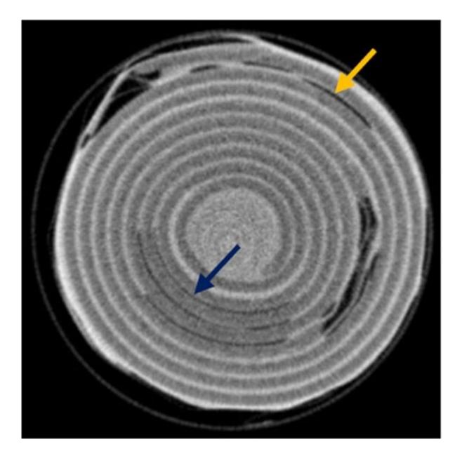
Neutrons can detect 'dry' regions (yellow arrow) where the elecrolyte is lacking. The blue arrow shows areas with a deficiency of Lithium. Credit: T.Arlt, I. Manke/HZB, R. Ziesche/UCL
