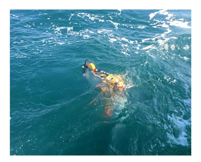
A Wirewalker, driven by waves and currents, sits at the ocean's surface during a field campaign led by oceanographers from the U.S. Naval Research Laboratory. The Wirewalker was equipped with a variety of instruments to measure light, conductivity, temperature, depth, light and acoustic backscatter, and dissolved oxygen throughout the water column. The NRL study was focused on
