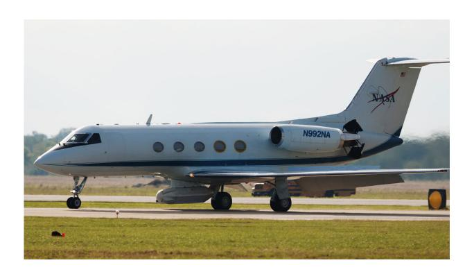
A Gulfstream III aircraft equipped with NASA's UAVSAR instrument, one of several instruments to be deployed for Delta-X. Credit: NASA
