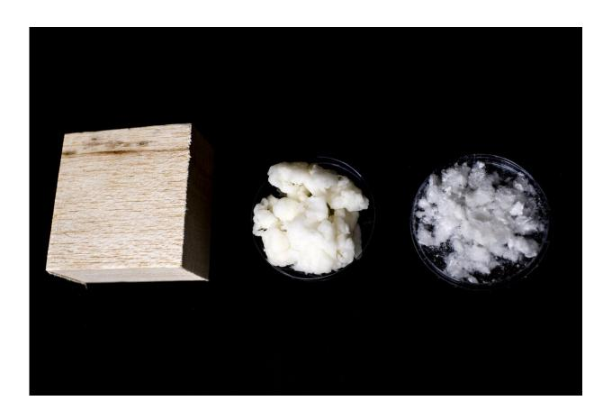
With cellulose from wood, Northeastern researchers have created a new biodegradable material to improve flow batteries and reduce the cost of storing energy from renewable sources. Credit: Ruby Wallau/Northeastern University
