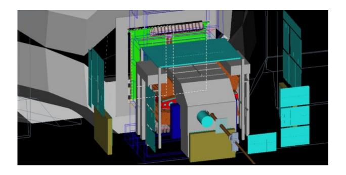
Illustration of the MoEDAL detector system (gold and light blue components), surrounding the LHCb experiment's VELO detector (central grey structure). Credit: CERN
