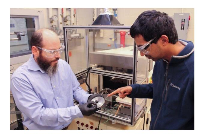
Army researchers Dr. Stephen Berkebile (left) and Nikhil Murthy (right) examine how silicon nitride responds to steel during dry sliding mechanical contact to better understand equipment breakdowns. Credit: Vincent Coburn
