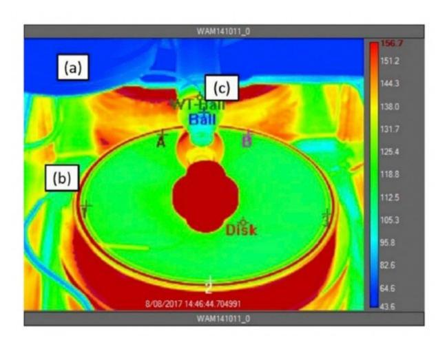
An infrared camera captures thermographic data of the ball-on-disk tribometer with labels indicating the locations of the (a) optical microscope objective, (b) disk thermocouple, and (c) ball thermocouple. Credit: Dr. Stephen Berkebile
