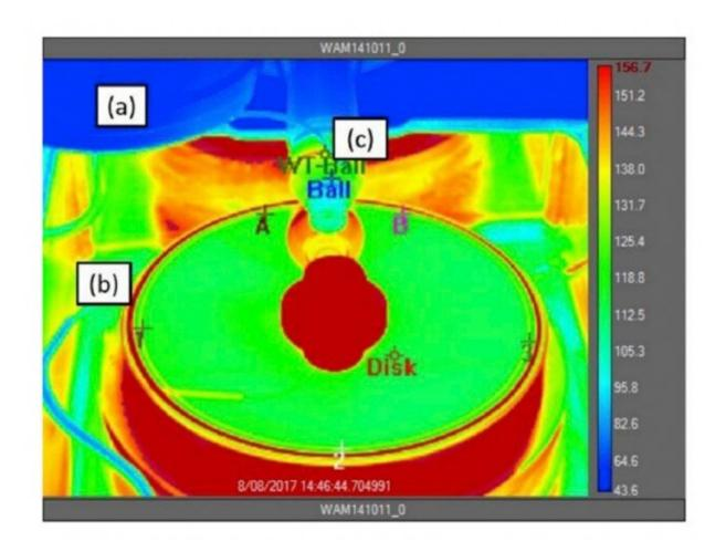
An infrared camera captures thermographic data of the ball-on-disk tribometer with labels indicating the locations of the (a) optical microscope objective, (b) disk thermocouple, and (c) ball thermocouple. Credit: Dr. Stephen Berkebile
