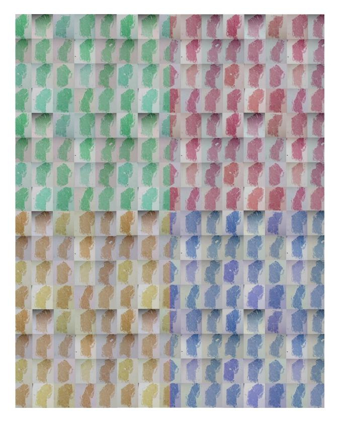
Atomically thin semiconductor wafers (MoS2 monolayers, lateral dimension of each panel ~ 1cm, wafer thickness of only ~0.7 nm). The researchers obtained
