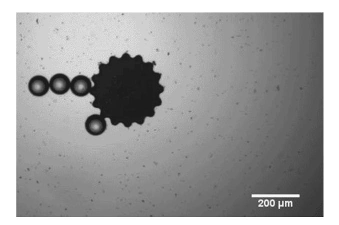
Shown in 4x speed, a flower-shaped microrobot approaches plastic beads, uses capillary forces to stick them to one of its petals, then releases them at the desired location by spinning in place. Credit: Penn Engineering
