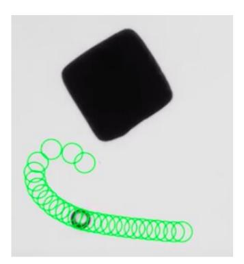
Particles are strongly attracted to the corners of square-shaped robots. The green outline shows the trajectory the particle takes as the robot approaches. Credit: University of Pennsylvania
