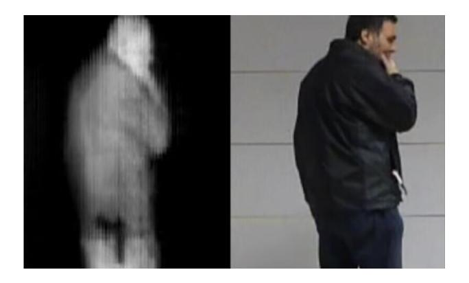
Terahertz radiation can be used for many kinds of imaging, such as in airports or in nondestructive materials testing. A new technique uses it for high-speed video. Credit: Sequestim/Cardiff University
