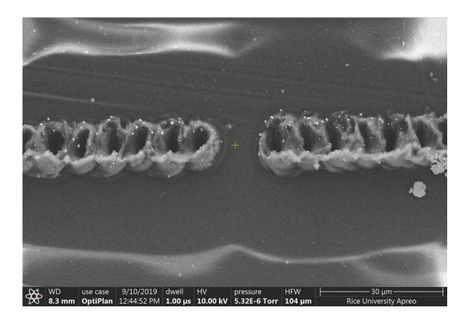
A scanning electron microscope image shows two traces of laser-induced graphene on a polyimide film. A laser mounted to the microscope was used to burn the patterns into the film. The technique shows promise for the development of flexible electronics. Credit: Tour Group/Rice University
