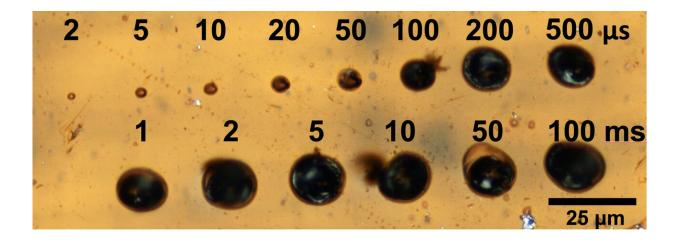
Scientists at Rice University and Oak Ridge National Laboratory used a small laser mounted to a scanning electron microscope to form dots and traces of conductive graphene on a polymer. The technique creates laser-induced graphene with features more than 60% smaller than the macro version and almost 10 times smaller than typically achieved with an infrared laser. Credit: Tour Group/Rice University
