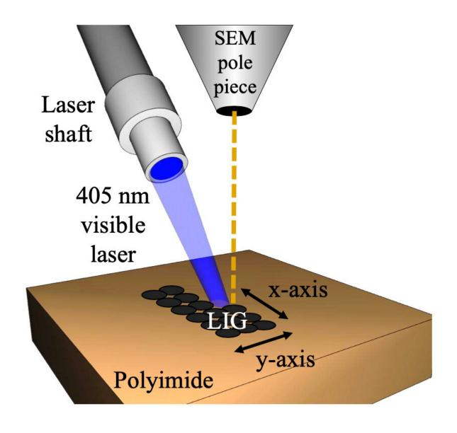
Scientists recorded the formation of laser-induced graphene made with a small
