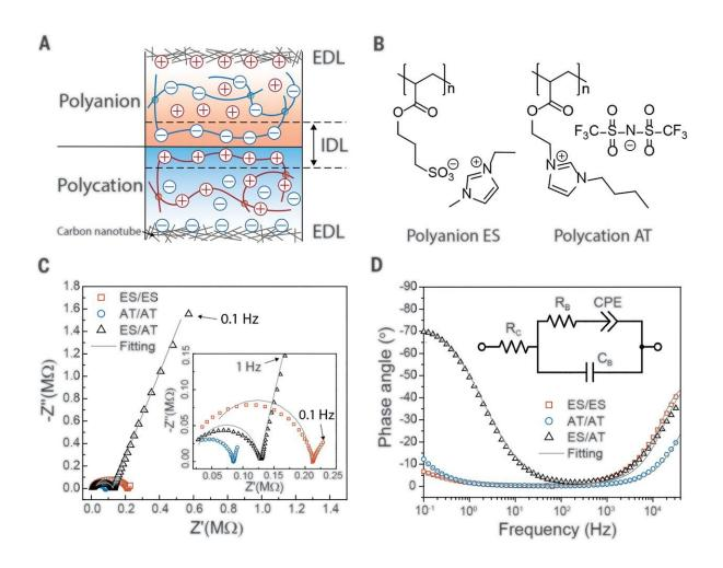
Formation of an IDL at the interface of two oppositely charged ionoelastomers. (A) Schematic illustration of a polyanion/polycation junction. High–surface area carbon nanotube electrodes are embedded within each ionoelastomer, resulting in low-impedance (high-capacitance) EDLs. (B) Chemical structures of the polyanion ES and polycation AT. (C) Nyquist plot and (D) Bode phase plot of acimpedance measurements. The inset in (C) shows an enlargement of the Nyquist
