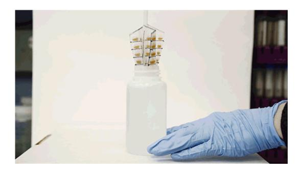
A whisk-like device lined with small pockets filled with gold polymer beads, fits inside a typical sampling bottle, and can be twirled to pick up any metal contaminants in water. Credit: Massachusetts Institute of Technology
