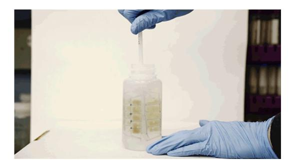
After the device is pulled out and dried, it can preserve any metal contaminants that it has picked up, for long periods of time. The device can be flattened and mailed to a lab, where the contaminants can be further analyzed. Credit: Massachusetts Institute of Technology
