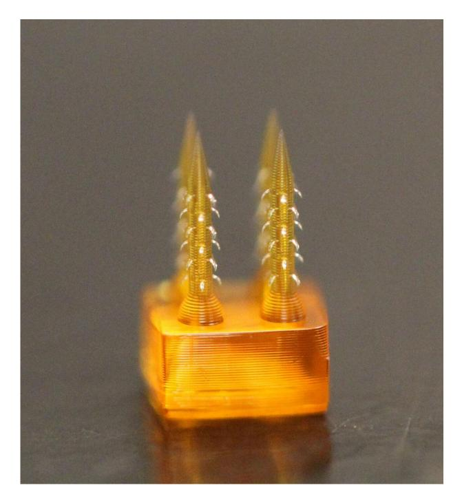
Microneedle array has backward-facing barbs that interlock with tissue when inserted, enhancing adhesion. Credit: Riddish Morde
