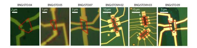
Graphene devices. Optical pictures of diverse samples. The red lines underline the edges of the hBN-encapsulated graphene flakes. Credit: Science, doi: 10.1126/science.aax8201
