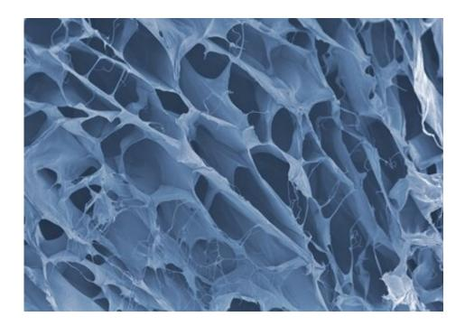
The novel biopolymer with mussel proteins exhibits a fine yet robust microstructure via scanning electron microscopy at 1000-fold magnification (colored). Credit: Empa
