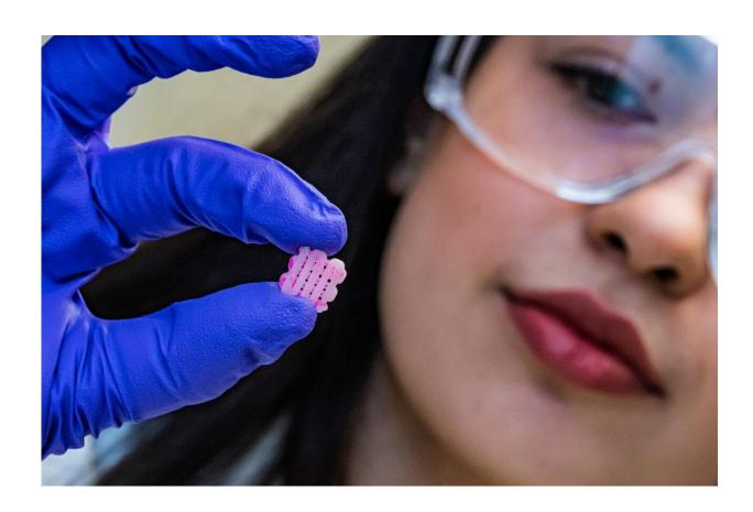
Rice University research scientist Maryam Elizondo holds a 3D-printed scaffold engraved with grooves for the deposition of live cells for implantation. The scaffold facilitates the growth of new tissues as it degrades. By protecting cells in grooves along the printed lines, Rice researchers designed the scaffold to enable different tissue-type layers within one scaffold. Credit: Jeff Fitlow/Rice University
