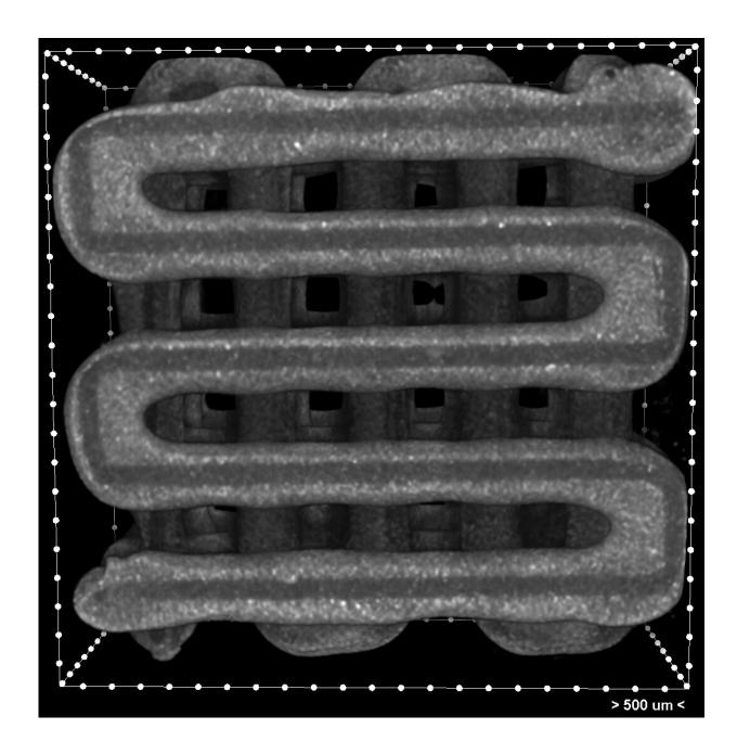
A microCT image shows a 3D-printed scaffold with clear grooves meant for the deposition of live cells. The grooved lines hold ink deposited during the printing process. Scaffolds can be made in any shape, based on medical images, to fill the site of a wound. Credit: Rice Biomaterials Lab
