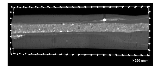
A microCT image shows a grooved thread that holds the low-viscosity bioink. They are part of a 3D-printed scaffold developed at Rice University to facilitate the growth of new tissue like bone and cartilage. The scaffolds degrade over time to leave layers of natural tissues in place. Credit: Rice Biomaterials Lab
