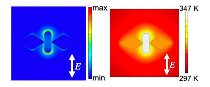
Calculated localized field (left) and temperature distribution (right) of the nanobutterfly structure. Credit: Fujiwara H., et al, Nano Letters. December 23, 2019
