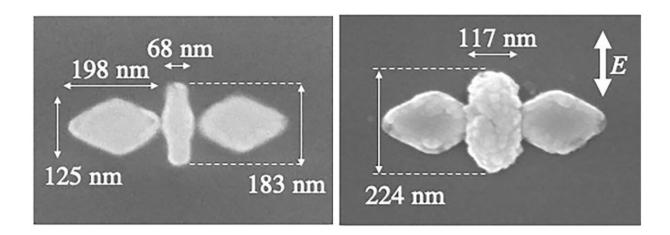
Scanning electron microscope images of the nano-butterfly structure before (left) and after (right) laser irradiation. Semiconductor zinc oxide has crystalized on the surface of the gold nanorod. Credit: Fujiwara H., et al, Nano Letters.
