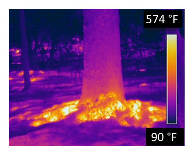
This infrared image shows that long-duration heating was most prominent where accumulated forest floor duff was deepest, particularly at the base of mature pines in long-unburned sites. Temperatures potentially lethal to plant tissues were sustained for several hours as deep as 4 inches near pines, and sustained temperatures high enough to impact soil nutrients were observed for up to 35
