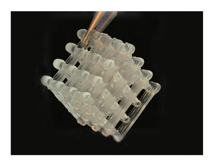
A 3D-printed hydrogel lattice contains yeast cells that can allow for the continuous production of ethanol. Credit: Cockrell School of Engineering, The University of Texas at Austin
