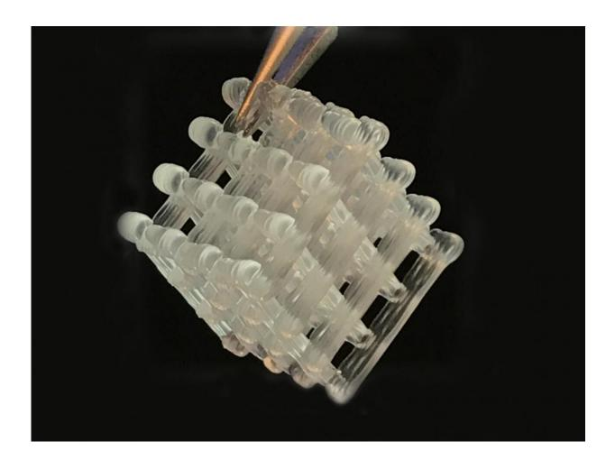
A 3D-printed hydrogel lattice contains yeast cells that can allow for the continuous production of ethanol. Credit: Cockrell School of Engineering, The University of Texas at Austin
