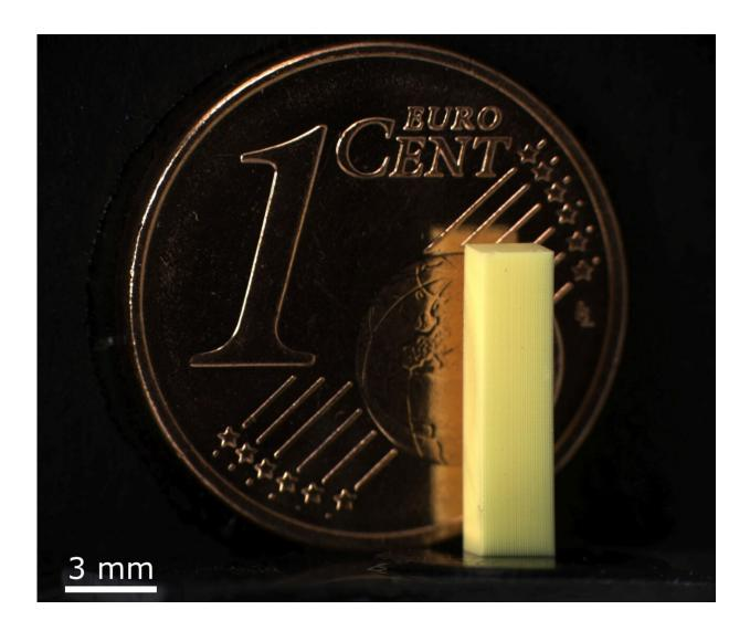
The metamaterial printed with the new system consists of a complex threedimensional lattice structure on the micrometer scale. Credit: Vincent Hahn, KIT
