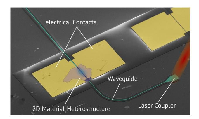
An electron microscope image of the ETH light detector with the thin layer of the two-dimensional heterostructure, the optical waveguide and the electrical contacts through which the signal of the detector is read out. Credit: ETH Zurich
