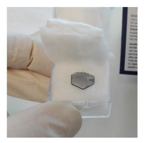
A molybdenum ditelluride crystal is shown. Wafer-thin layers of the crystal can be combined with two graphene layers to make up a vertical heterostructure. Credit: ETH Zurich
