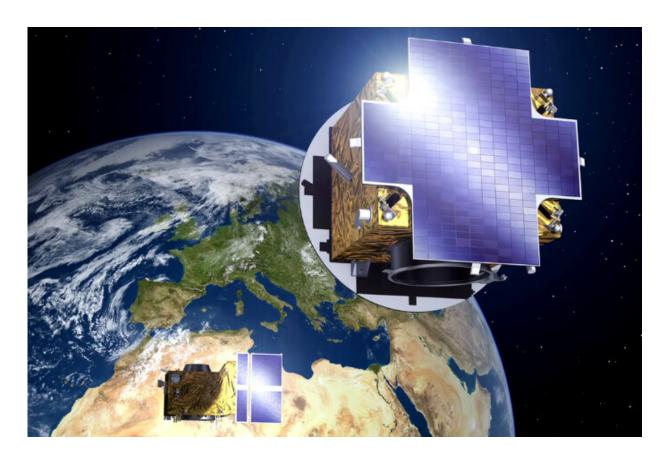
Proba-3's pair of satellites will be in a highly elliptical orbit around Earth, performing formation flying manoeuvres as well as scientific studies of the solar corona. The occulter satellite will have solar panels on its sun-facing side. Credit: ESA-P. Carril
