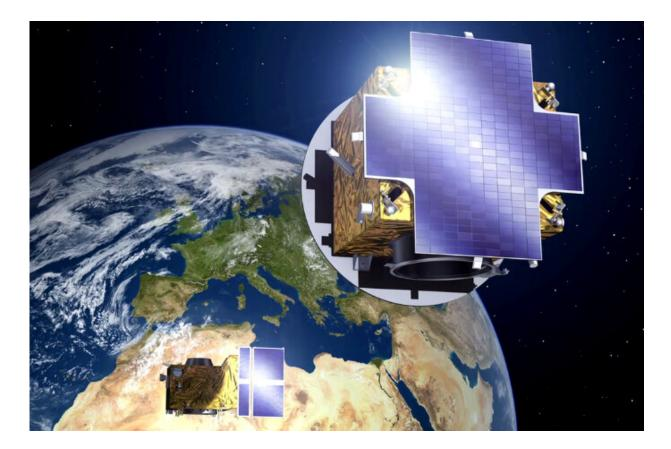
Proba-3's pair of satellites will be in a highly elliptical orbit around Earth, performing formation flying manoeuvres as well as scientific studies of the solar corona. The occulter satellite will have solar panels on its sun-facing side. Credit: ESA-P. Carril
