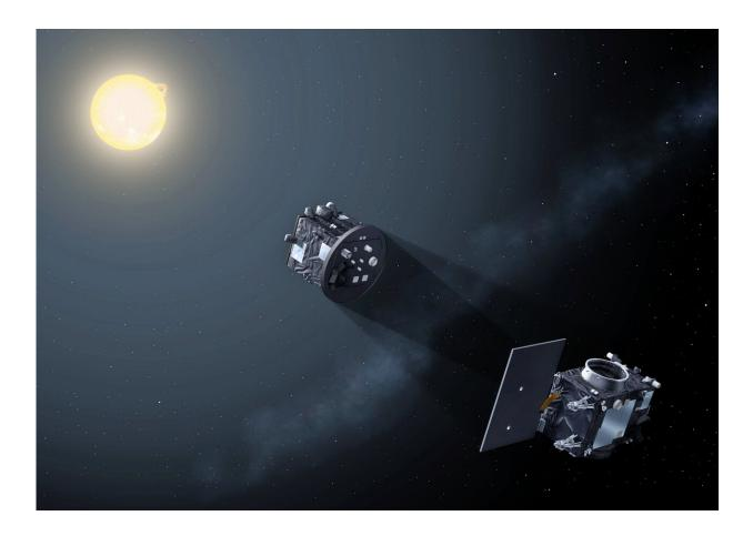
Due to launch together in 2020, the two satellites making up Proba-3 will fly in precise formation to form an external coronagraph in space, one satellite eclipsing the Sun to allow the second to study the otherwise invisible solar corona. Credit: ESA
