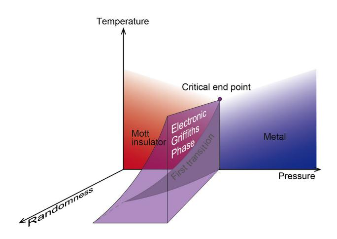
Schematic temperature-pressure-randomness phase diagram of the Mott transition system examined by the researchers. The electrons in the electronic Griffiths phase behave like soft matter. Credit: Yamamoto et al.
