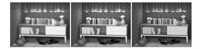
In the left image, the basketball in front is in focus. In the center image, the storage unit is in focus. The right image shows an all-in-focus image from reconstructed light field data. Credit: University of Michigan
