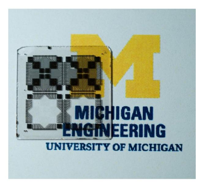
Four fabricated photodetectors resting on a sheet of paper to illustrate the high degree of transparency. The top two devices have a transparent window size of  $200 \times 200 \ \mu m^2$ , and the bottom two have a window size of  $5 \times 5 \ mm^2$ .
