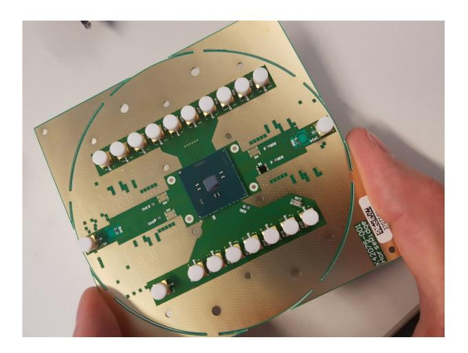
Horse Ridge mounted on the board ready to be installed in the cryogenic refrigerator. Credit: QuTech
