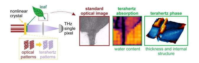
The time-resolved nonlinear ghost imaging camera uses a nonlinear crystal to convert standard laser light to terahertz patterns, allowing the reconstruction of complex samples using a single terahertz pixel. Credit: University of Sussex
