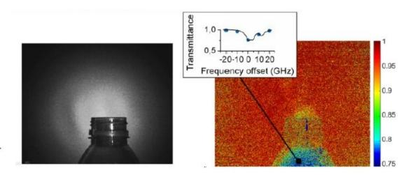
The researchers used their new direct hyperspectral dual-comb imaging approach to acquire hyperspectral images of ammonia gas escaping from a bottle. The left image shows a photograph of the scene while the right image shows a map of ammonia transmittance extracted from a single interferogram. The inset shows the spectral response measured by the system at a particular pixel. Credit: Pedro Martín-Mateos, Universidad Carlos III de Madrid
