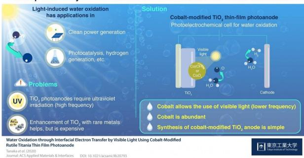
Cheap and easy enhancement of photoanodes for water oxidation. Credit: Tokyo Institute of Technology
