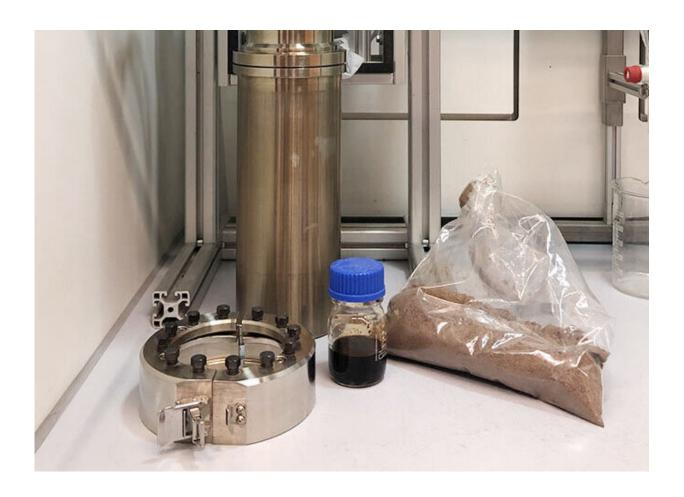
This picture displays the chemical reactor used in the study to split wood into wood pulp and lignin oil. Credit: KU Leuven
