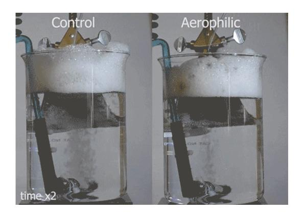
In two identical beakers with a constant stream of bubbles, inserting a piece of the new textured material developed by the MIT team (on right) causes the foam buildup at the top of the beaker to dissipate almost completely, whereas a similar material without the special surface texture (at left) leaves the foam unidisturbed. Credit: Varanasi Lab
