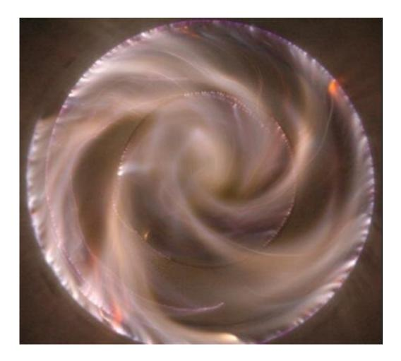
Using a gliding arc plasmatron, Drexel University researchers can create a vortex of cold plasma with enough energy to break apart PFAS compounds in water. Credit: Drexel University
