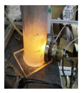
Gliding arc plasmatron, developed at Drexel University, is being used to eliminate PFAS contamination from drinking water. Credit: Drexel University
