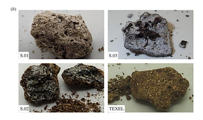
Details for ambergris samples analysed. (a) Map showing localities where ambergris samples were originally found. (b) Photographs showing high diversity in physical characteristics of ambergris fragments: TEXEL151212 (from dissected whale specimen) was grainy in consistency, while jetsam samples superficially appeared more dense and heterogeneous, and were internally equigranular and significantly paler in colour. Credit: *Biology Letters* (2020). DOI: 10.1098/rsbl.2019.0819
