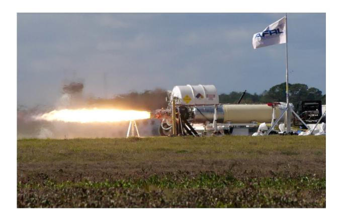
A recent X-60A hot fire test, conducted at Cecil Spaceport in Jacksonville, Florida. The X-60A, developed through an Air Force Research Laboratory Small Business Innovation Research contract, is an air-launched rocket designed for hypersonic flight research. Credit: U.S. Air Force
