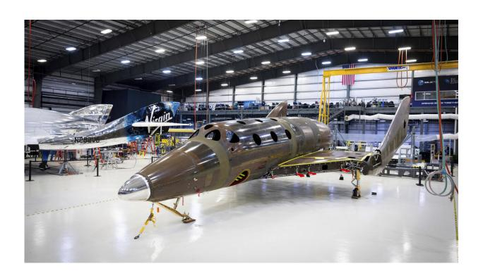
This photo released by Virgin Galactic Wednesday, Jan. 8, 2020, shows Virgin Galactic's next passenger spaceship standing on its landing gear in what is known as a weight-on-wheels test, in a hangar at the company's Mojave Air & Space Port in Mojave, Calif. Continuing work on the new ship includes connecting flight control and other integrated systems. The company anticipates commercial flights this year at Spaceport America in southern New Mexico. (Thomas Storesund/Virgin Galactic via AP)
