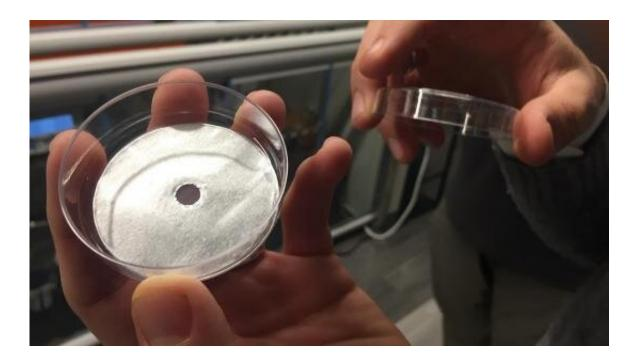
Researchers developed this highly permeable perfluorinated sulfonic acid ionomer that can improve performance of hydrogen fuel cells. Credit: NYU Tandon School of Engineering
