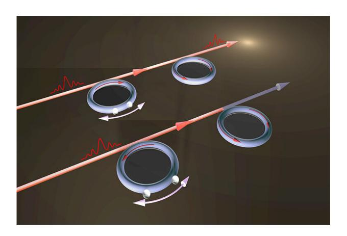
Electromagnetically induced transparency (EIT) is 'tuned' by two particles on the optical resonator. The different locations of particles control the propagation of light in either clockwise or counterclockwise directions, which switch on (upper configuration) or off (lower configuration) the interference of light, leading to controllable brightness (EIT) and darkness in the output. Credit: Yang Lab
