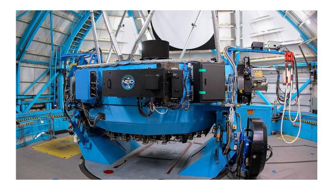
The NEID instrument, mounted on the 3.5-meter WIYN telescope at the Kitt Peak National Observatory. The NASA-NSF Exoplanet Observational Research (NN-EXPLORE) partnership funds NEID (short for NN-EXPLORE Exoplanet Investigations with Doppler spectroscopy). Credit: NSF's National Optical-Infrared Astronomy Research Laboratory/KPNO/NSF/AURA
