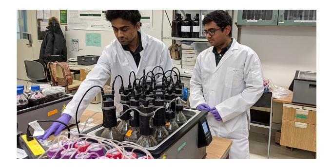
Environmental engineering master's student Bappi Chowdhury (left) and supervisor Bipro Dhar in the lab with a "digester" they are developing that uses microbes to convert a mixture of food waste and fat, oil and grease into renewable biomethane. Credit: Sean Townsend
