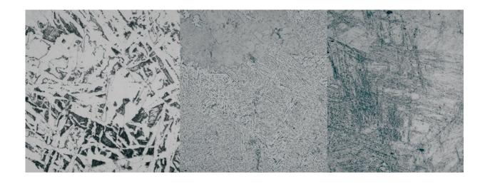
The three types of alloy microstructures identified in microscopic images. From left to right: Ferrite/Pearlite, Ferrite/Pearlite/Bainite and Bainite/Martensite. Credit: NIMS
