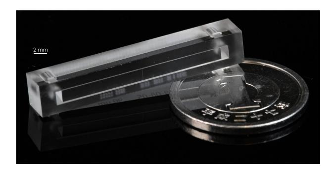
A photograph of a glass microchannel. One of the side walls has been removed to expose a slender glass microcylinder in the center of the channel. 1-yen coin included for scale. Credit: Okinawa Institute of Science and Technology
