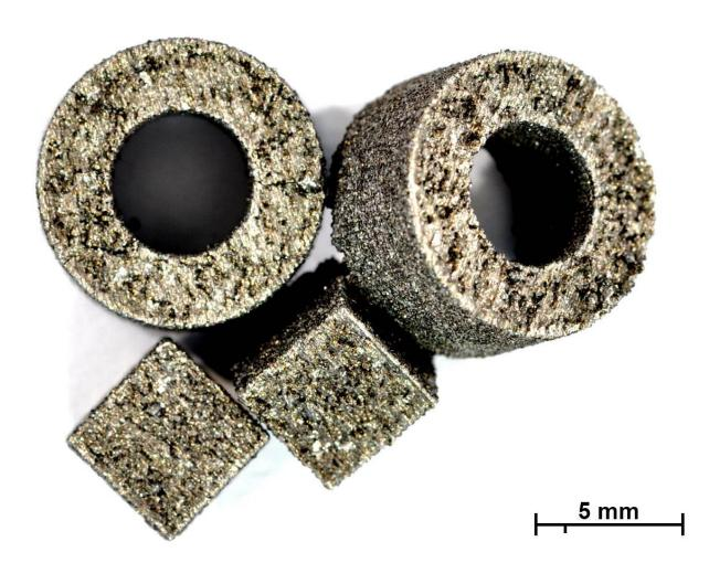
At Graz University of Technology, miniaturised supermagnets were produced for the first time using laser-based 3D printing. Credit: IMAT – TU Graz
