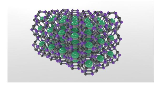
Carnegie's Tim Strobel and Li Zhu led a team that used advanced structure searching tools to predict the first thermodynamically stable carbon-based clathrate and then synthesized the clathrate structure, which is comprised of carbon-boron cages that trap strontium atoms. Credit: Tim Strobel.
