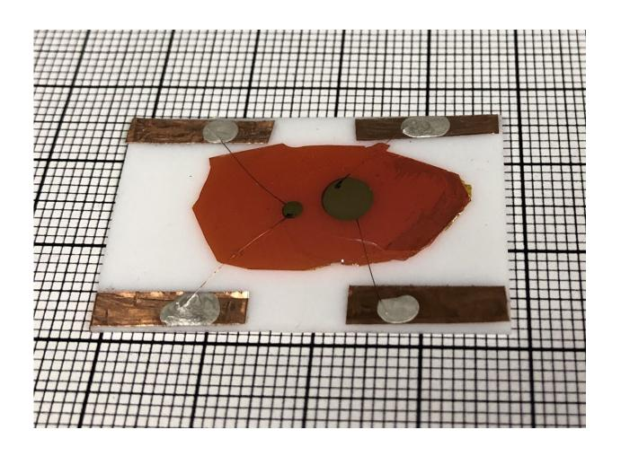
A prototype of a working, pocket-sized neutron detector made with a high lithium-containing material. Credit: Northwestern University/Argonne National Laboratory
