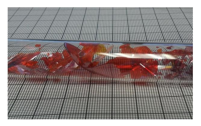
New material (lithium-indium-phosphorous-selenium) is lithium-rich, making the semiconductor neutron detector possible. Credit: Northwestern University/Argonne National Laboratory
