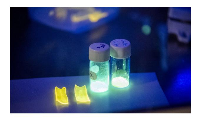
On the left are two films of the polymer, with the copper complexes incorporated as cross-linkers. On the right are two vials of the isolated copper complexes, which were developed by Pradyna Patil, a former postdoctoral scholar. The polymer films and isolated copper complexes luminesce under ultraviolet light. Credit: Okinawa Institute of Science and Technology
