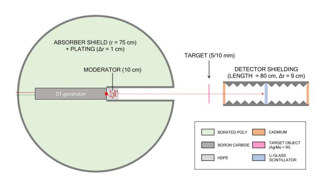
The schematic of a compact neutron resonance transmission analysis platform using a deuterium-tritium source (not to scale), shielding, a moderator for slowing down the neutrons to the eV regime and a boron-lined collimator. Credit: Ezra M. Engel and Ethan A. Klein, MIT
